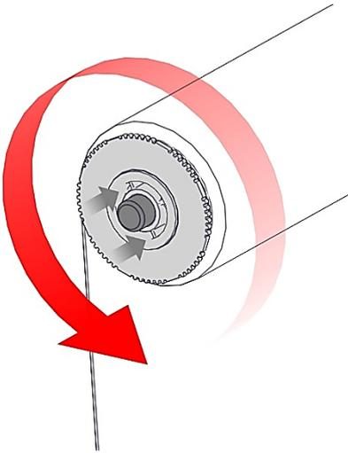
NOTE: Retract Idler Pin by rotating counter-clockwise
