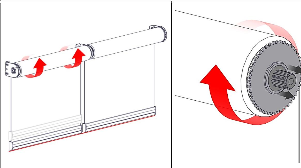
NOTE: Rotate fabric/tube until weight bars are in line
