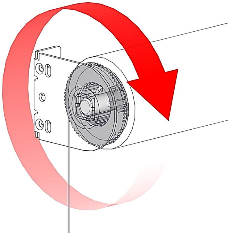
NOTE: Extend the Idler Pin by rotating clockwise, Ensure pin is fully extended through Bracket
