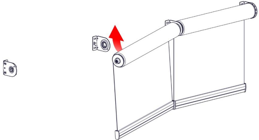
NOTE: Ensure weight bars are at even heights when installing Shade “A”
