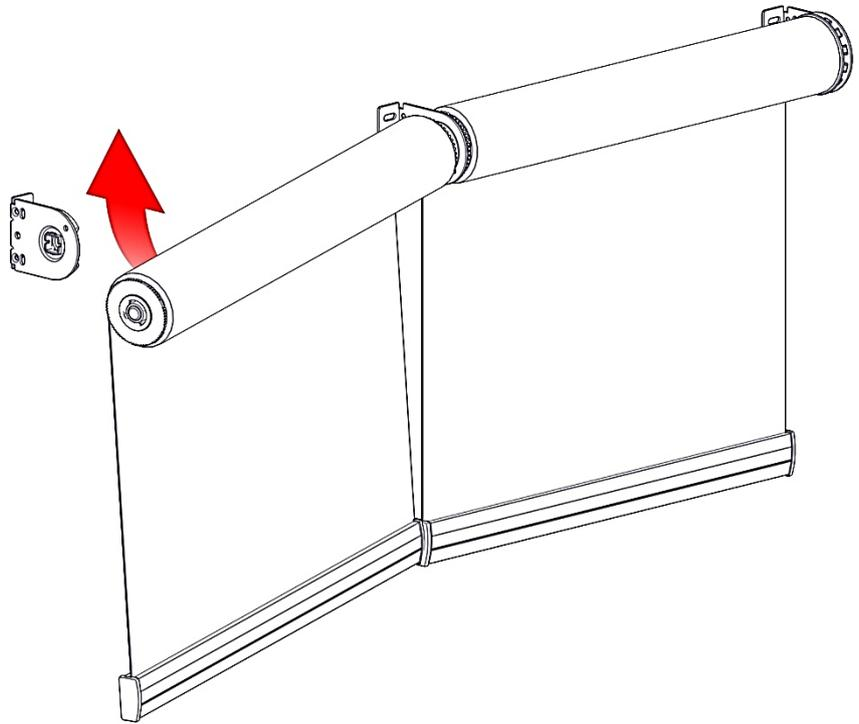
NOTE: Ensure weight bars are at even heights when installing Shade “A”
