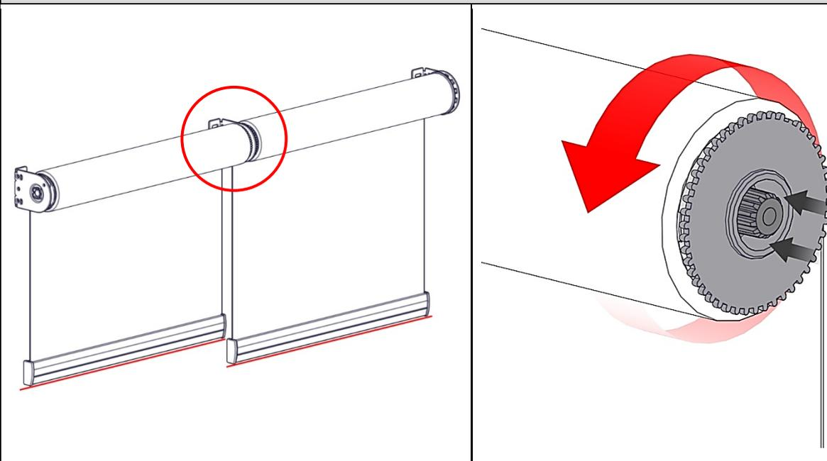
NOTE: Rotate Male Easy-Link Wheel counter clockwise to retract the pin connection
