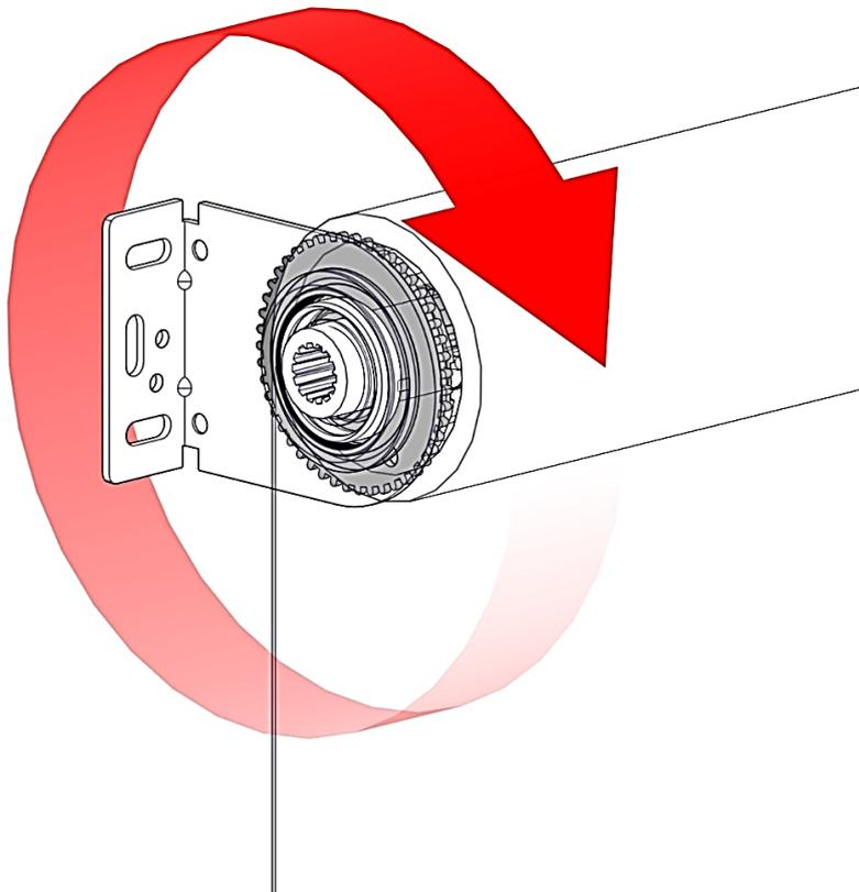
NOTE: Extend the female Easy-Link by rotating clockwise, Ensure pin is fully extended through Easy-Link Bracket
