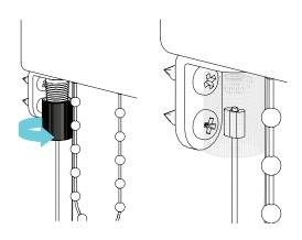
STEP 7. - PASS THE WIRE THROUGH THE BOTTOM RAIL WIRE GUIDE END CAP
