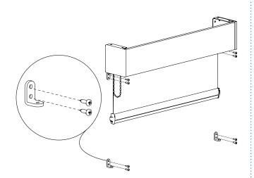
STEP 2. - SCREW THE TENSION ADJUSTER TO THE TENSION STOPPER
