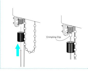
STEP 5. - CRIMP THE TOP CLIP USING A CRIMPING TOOL
