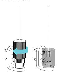
STEP 11. - ADJUST THE WIRE TENSION BY ROTATING THE TOP AND BOTTOM TENSION ADJUSTER COVERS
