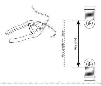
STEP 4. - PASS THE WIRE THROUGH THE TENSION ADJUSTER COVER AND CRIMPING CLIP
