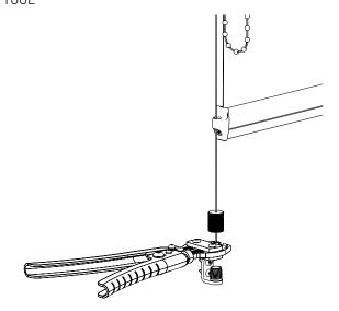
STEP 10. - ROTATE THE TENSION ADJUSTER COVER IN CLOCKWISE DIRECTION
