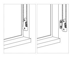
Can be installed with screws or industrial grade adhesive.
