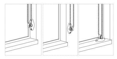
Can be installed with screws or industrial grade adhesive.
