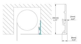
For use with bottom closures to hide recessed shades without the need for installing a pocket
